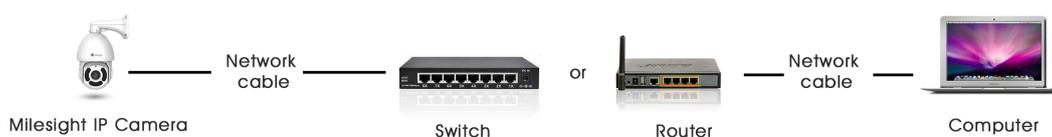
Figure 2-1-2 Connect via a switch or a Router
