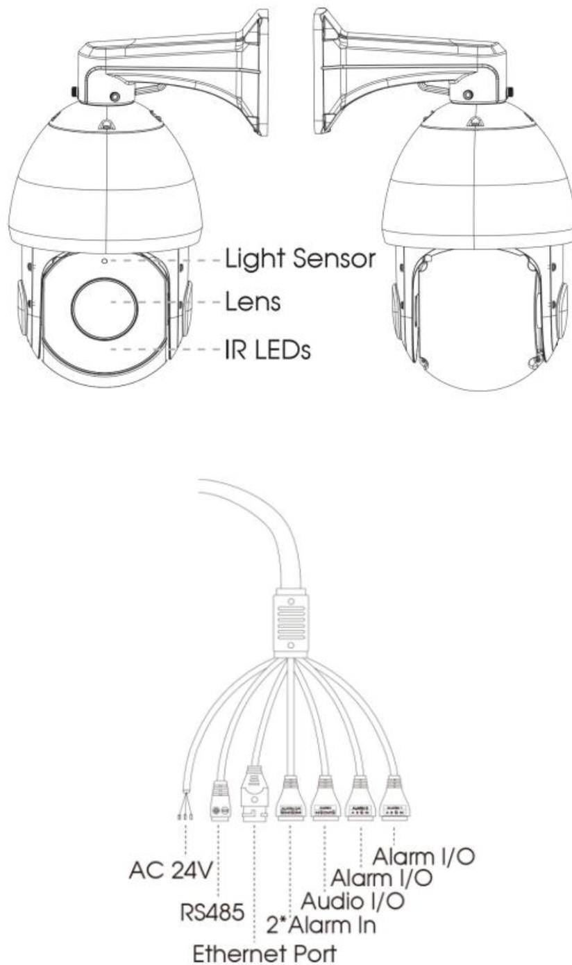
Figure 1-3-2 AI 23X/30X/36X/42X Speed Dome Network Camera
