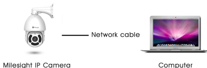
Figure 2-1-1 Connect the camera to the PC directly
