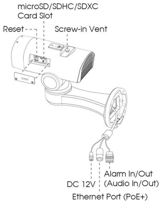
Figure 1-3-3 12X Mini PTZ Bullet Network Camera
