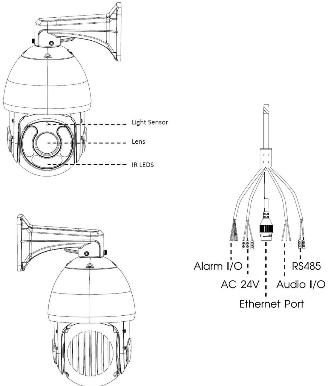
Figure 1-3-1 23X/30X/36X/42X Speed Dome Network Camera
