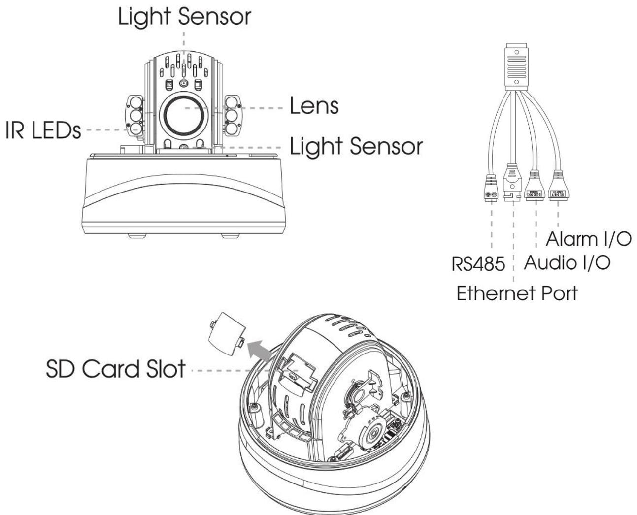
Figure 1-3-4 (AI) 12X/20X/23X Mini PTZ Dome Network Camera
